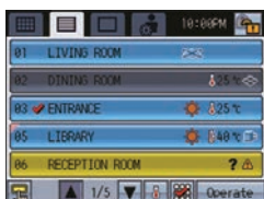
LIST screen Displays the detailed operation status of each group with group name.
