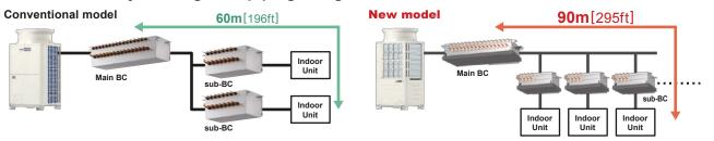
The piping length from the main BC controller to indoor units has been increased from 60m[196ft] to 90m[295ft], providing greater flexibility in piping design.
